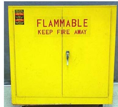
The bottom, top, door, and sides of metal cabinets shall be at least No. 18 gage sheet metal and double walled with 1½-inch air space. The door shall be provided with a three-point lock, and the door sill shall be raised at least 2 inches above the bottom of the cabinet.
